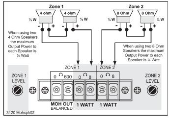
Fig 27A - Using two 4 or 8 ohm Speakers
